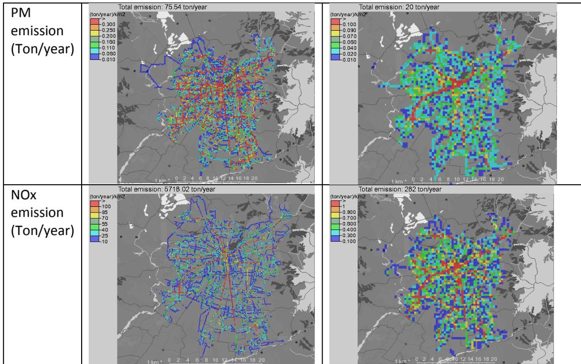
Modeling of before-and-after bus technology impact on PM and NOx emissions in Santiago with Euro III and Euro VI technology for standard buses (15-18 ton)
