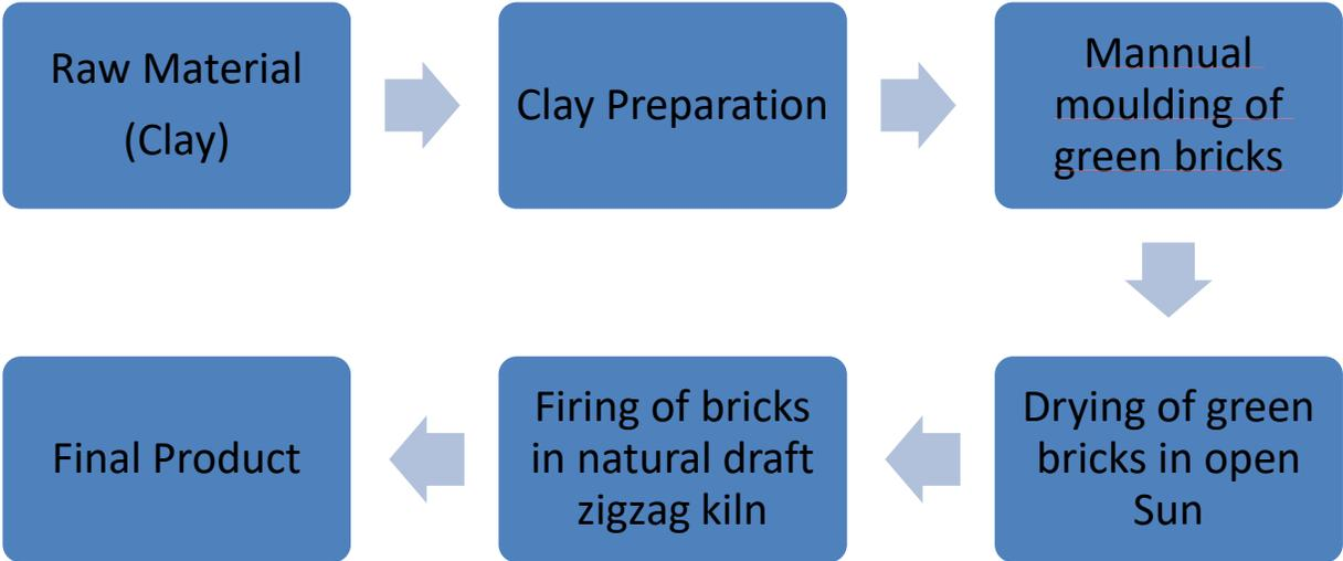
Figure 2: Schematic of brick production process at the Natural Draft Zigzag Kiln
