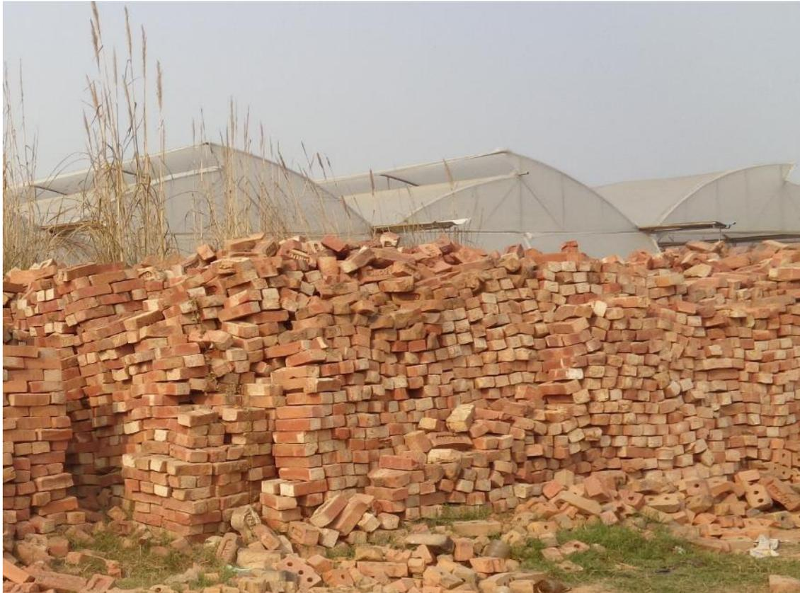
Figure 1: A lot of flyash-clay bricks stacked after firing (finished product)
