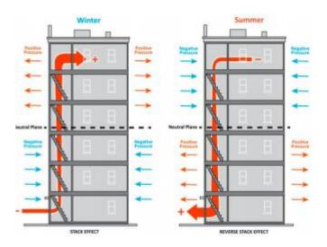
b. Building Stack Effect Solution: pressurization in the lobby to reduce the stack effect. An exhaust system is recommended to keep the home below the pressure in the corridor or hallway, this ensures that a contaminant from one apartment would never enter another. Open windows should also be minimized to meet minimum ventilation requirements.
