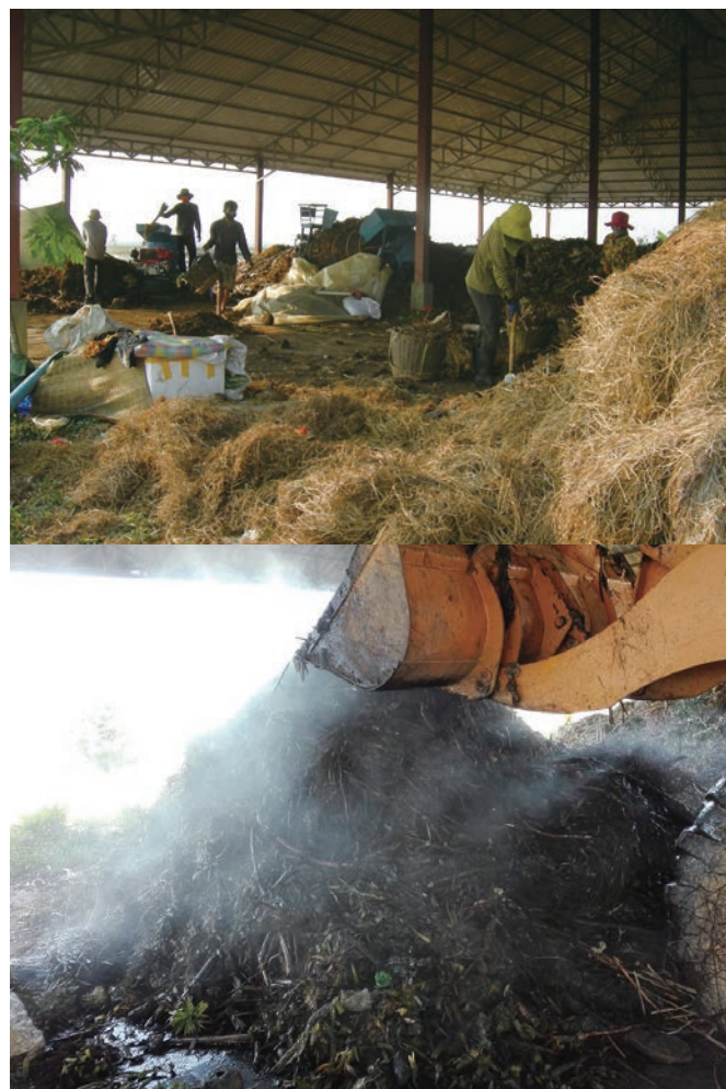
Figure 12: Windrow Composting of Organic Waste
