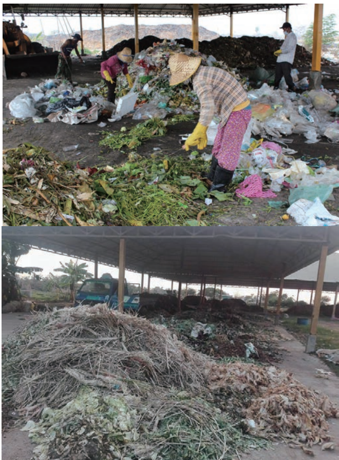
Figure 16: Improved Quality of Organic Waste Delivered to Composting Facility (Before - up, After - down)
