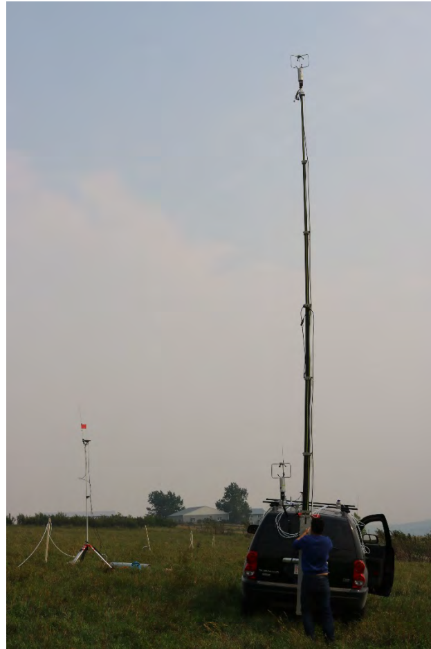
9 m tall mast with 8 sampling channels
