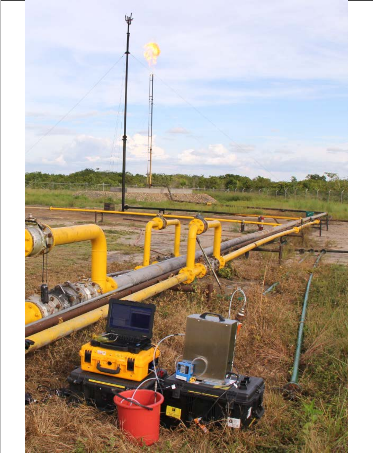
Figure 4: Photographs of the flare at CCAC.3 Battery with the tracer test in progress in the foreground, 7 August 2015.
