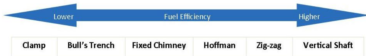
Figure 6. Relative fuel efficiencies for various brick kiln technologies assuming good operating practices.* Source: Compiled from the presentation of D.J. Reeve [28].
