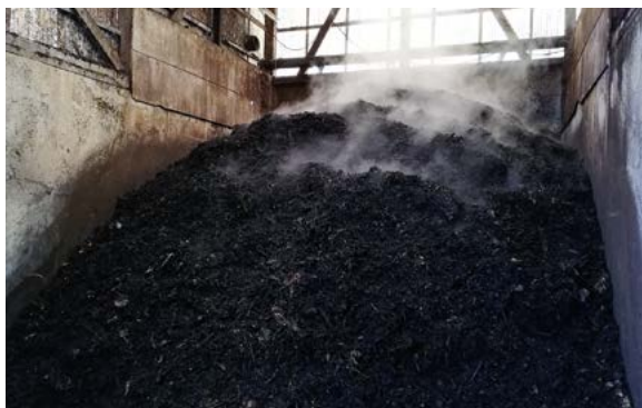
Fig. 25 Primary aerobic fermentation process in Osaki Town, Japan
