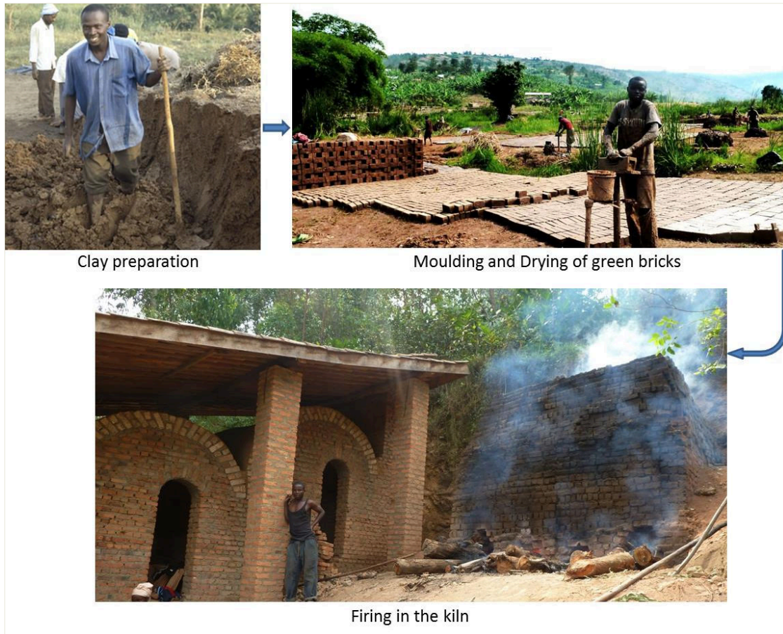
Figure 1: Brick making process
