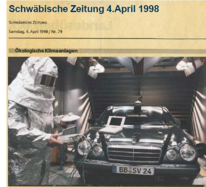
...the greenhouse gas effect of the car AC system can be cut by a third when applying carbon dioxide as a refrigerant
