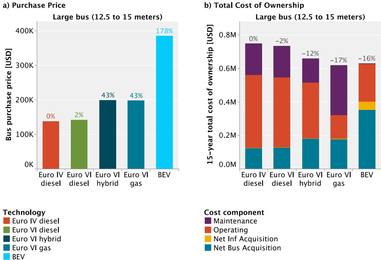
Figure 4. The effect of cost perspective on affordability of soot-free urban buses. (A) Decisions based on purchase price alone put cleaner and more efficient technology further out of reach. (B) Total cost of ownership flips the cost calculus, suggesting the most efficient soot-free technologies are the least expensive to acquire and operate since they provide fuel savings that pay for higher up-front costs. Euro VI gas includes compressed natural gas only.
