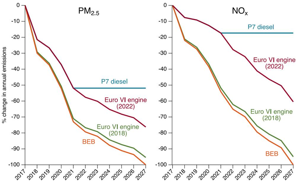
Figure 3. Annual change in PM<sub>2.5</sub> and NO<sub>x</sub> emissions for soot-free engine technologies compared with baseline P-7 (Euro V) diesel technology. The difference between zero emission battery-electric and Euro VI diesel engines is comparatively small over the course of 10 years.
