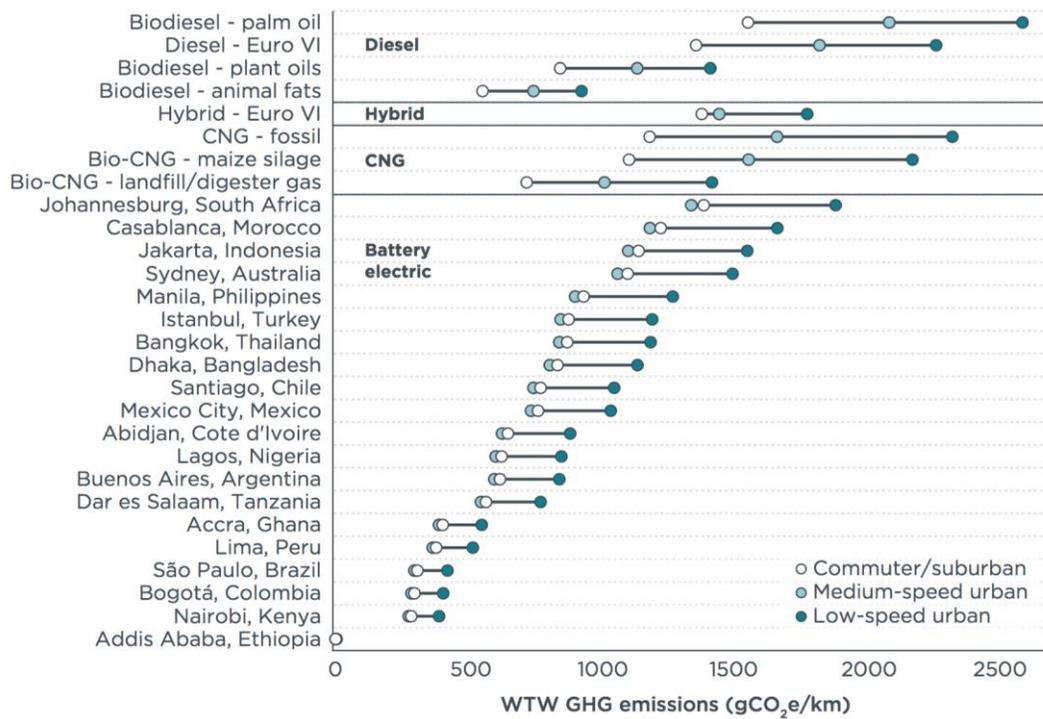
Figure 3. Well-to-wheel greenhouse gas emissions of soot-free engines in 20 targeted cities. Battery –electric arranged in order of highest to lowest carbon intensity by city and compared against diesel, diesel-hybrid, and gas engines. Effect of commuter, medium-speed, and low-speed driving conditions included.
