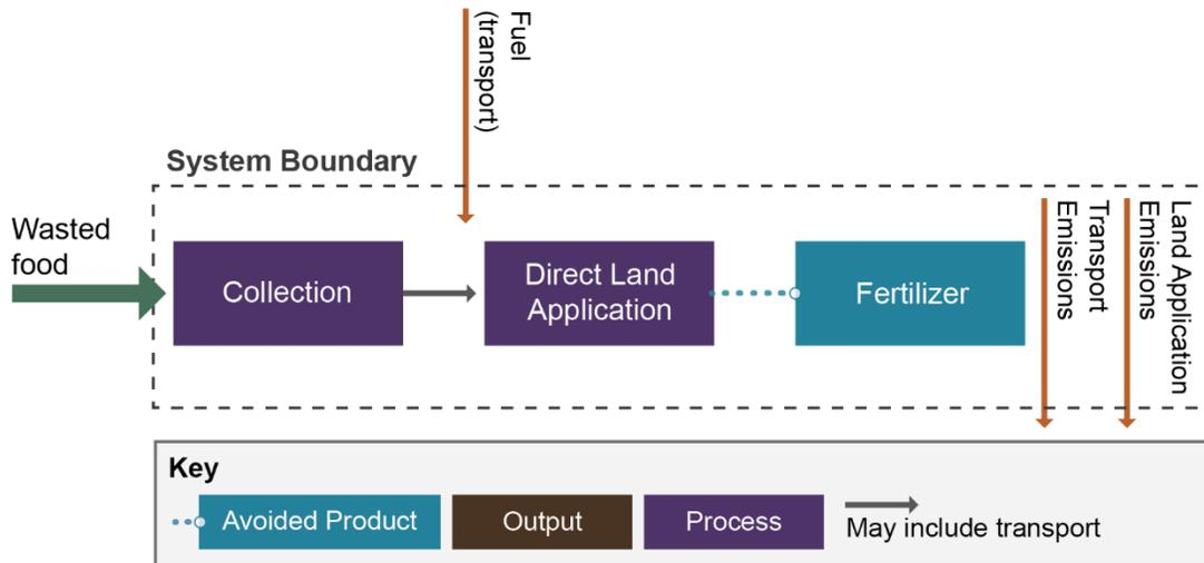
**FIGURE 2-9. DIAGRAM OF DIRECT LAND APPLICATION OF WASTED FOOD**
