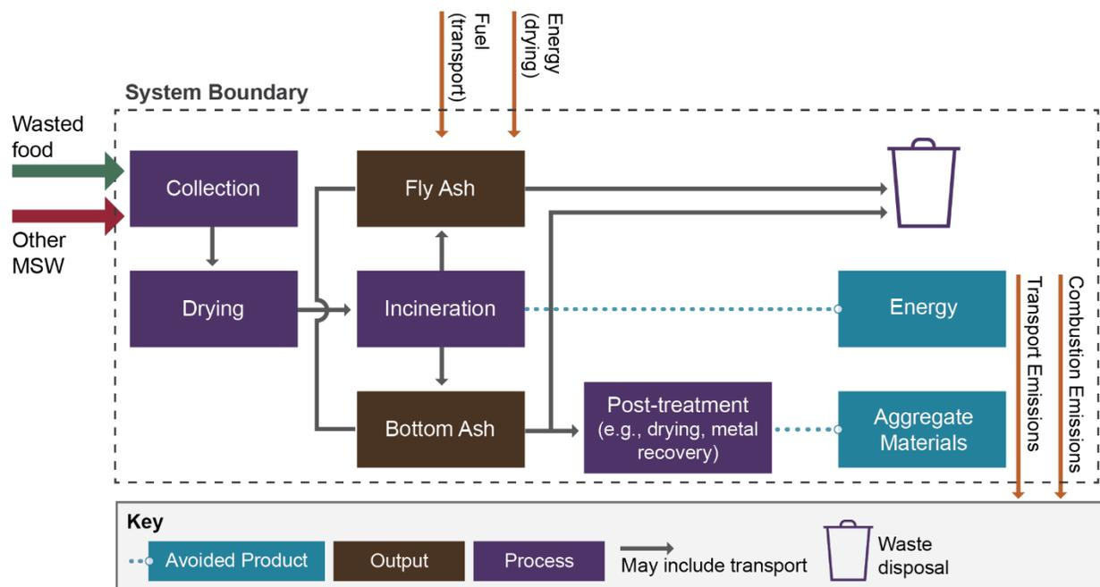
**FIGURE 2-8. DIAGRAM OF CONTROLLED COMBUSTION OF WASTED FOOD (AS PART OF MSW) WITH ENERGY RECOVERY**
