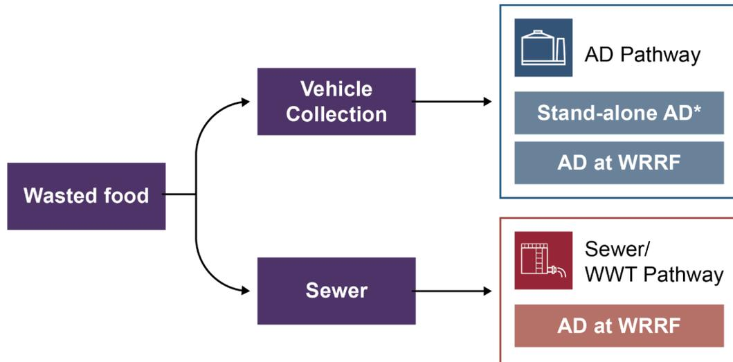
**FIGURE 2-4. DIAGRAM DISTINGUISHING ANAEROBIC DIGESTION AND SEWER/WWT PATHWAYS**
