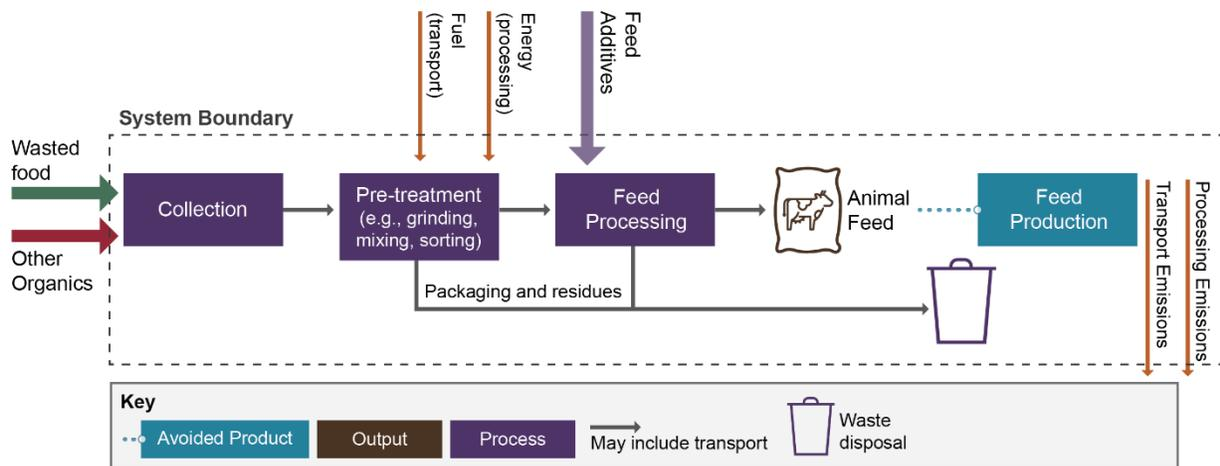
**FIGURE 2-6. DIAGRAM OF WASTED FOOD CONVERSION TO ANIMAL FEED**
