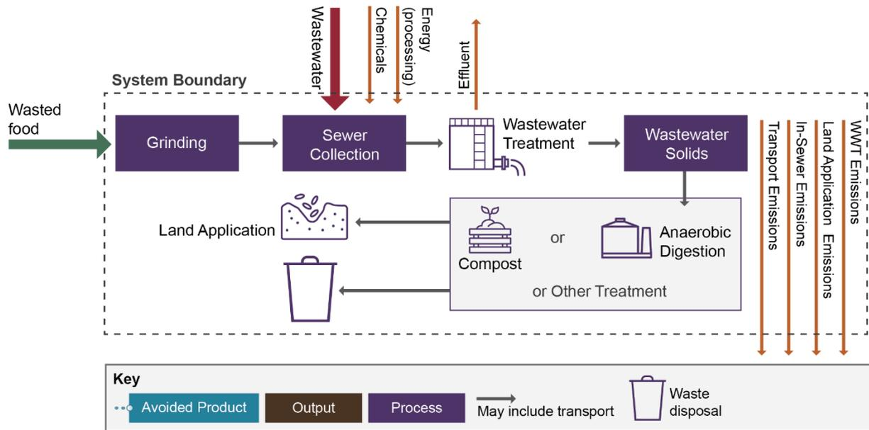
**FIGURE 2-11. DIAGRAM OF WASTED FOOD PROCESSING VIA SEWER/WASTEWATER TREATMENT**
