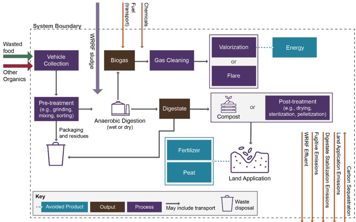
**FIGURE 2-5. DIAGRAM OF ANAEROBIC DIGESTION AND CO-DIGESTION OF WASTED FOOD**
