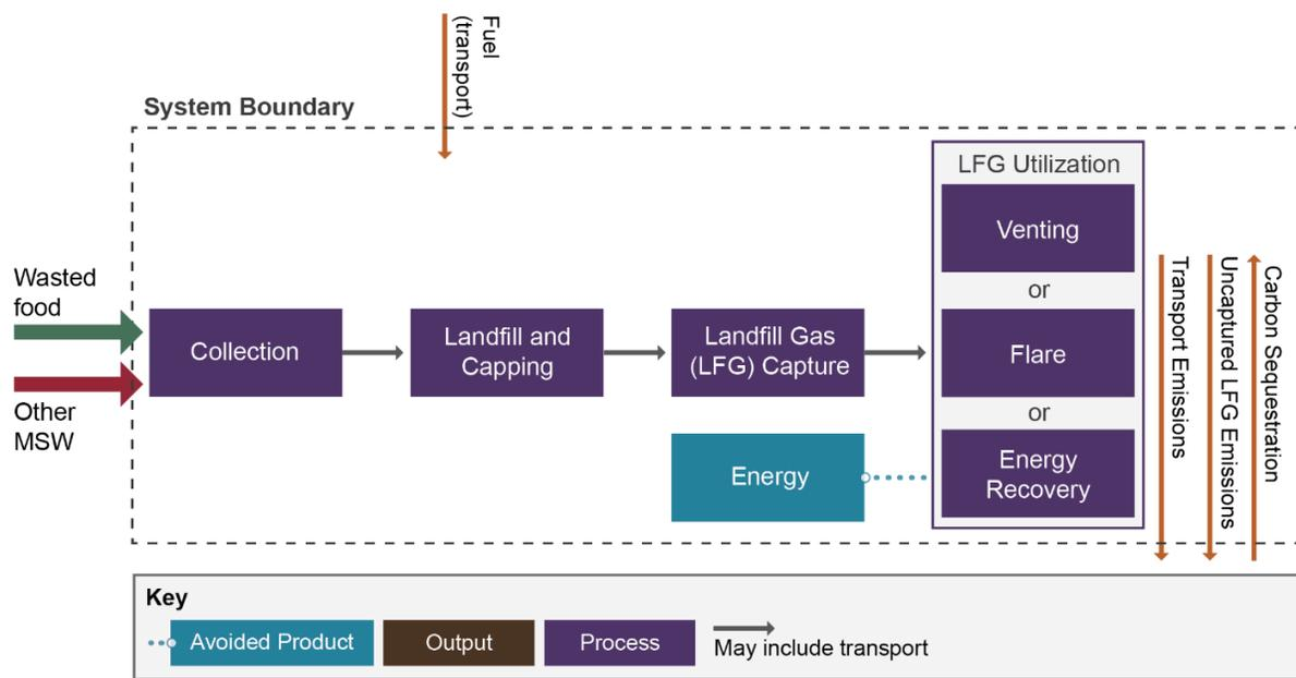
**FIGURE 2-10. DIAGRAM OF WASTED FOOD LANDFILLING WITH ENERGY RECOVERY**
