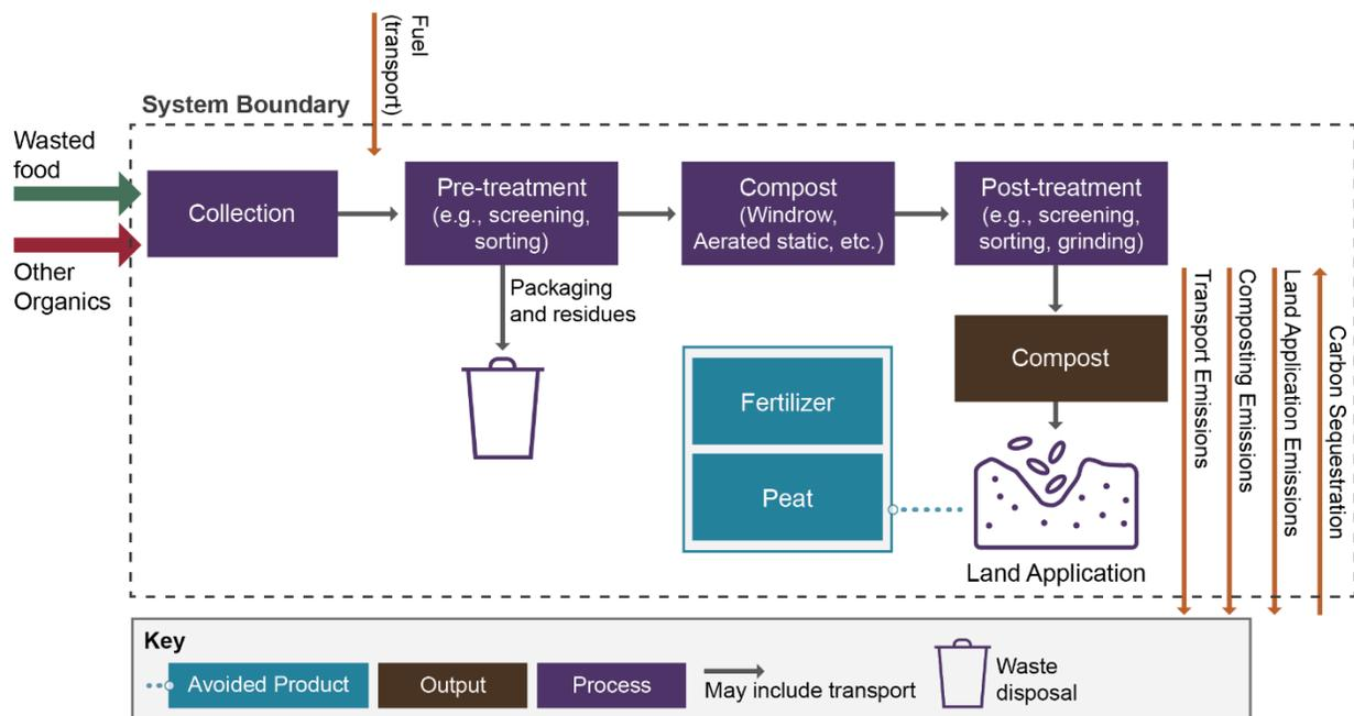
**FIGURE 2-7. DIAGRAM OF WASTED FOOD COMPOSTING, INCLUDING A PROMINENT CO-WASTE SUCH AS MUNICIPAL GREEN WASTE**
