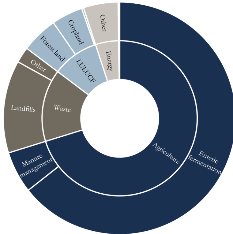
Figure 2. Total methane emissions in Sweden 2020 (4.55 Mt CO 2 -eq. including LULUCF). Methane emissions from the IPPU sector are excluded in this figure due to the small amount compared to the total level of methane emissions in Sweden. Total methane emissions in the agriculture sector amounted to 3.2 Mt CO 2 -eq (enteric fermentation 2.93 Mt CO 2 -eq and 0.26 Mt CO 2 -eq in manure management). Total methane emissions in the waste sector amounted to 0.68 Mt CO 2 -eq (0.58 Mt CO 2 -eq in landfills and 0.1 Mt CO 2 -eq in other). For the LULUCF sector, total methane emissions amounted to 0.44 Mt CO 2 -eq (0.23 Mt CO 2 -eq forest land and 0.2 Mt CO 2 -eq in crop land). Total methane emissions in the energy sector amounted to 0.20 Mt CO 2 -eq and mainly consists of emissions from energy industries, manufacturing industries, transport, and stationary combustion (in this figure these categories are included as Other).
